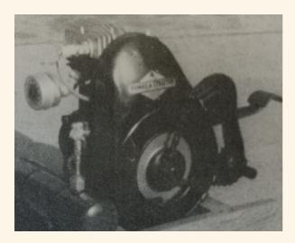
A: We're not sure that the Maytag engines were horsepower rated – their primary duty was to run the washing machines that Maytag built. However, it is possible to calculate the approximate delivered brake horsepower by the formula:
